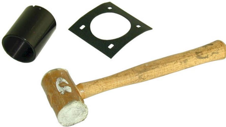
Using a curved surface and soft mallet, place the correct curve in the backup plate to match the curve in the optical tube. (With Sonotube installations you may wish to place an additional backup plate on the inside of the optical tube.)
