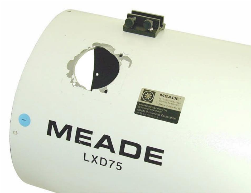
Using the wrench, punch the larger hole in the optical tube assembly.
