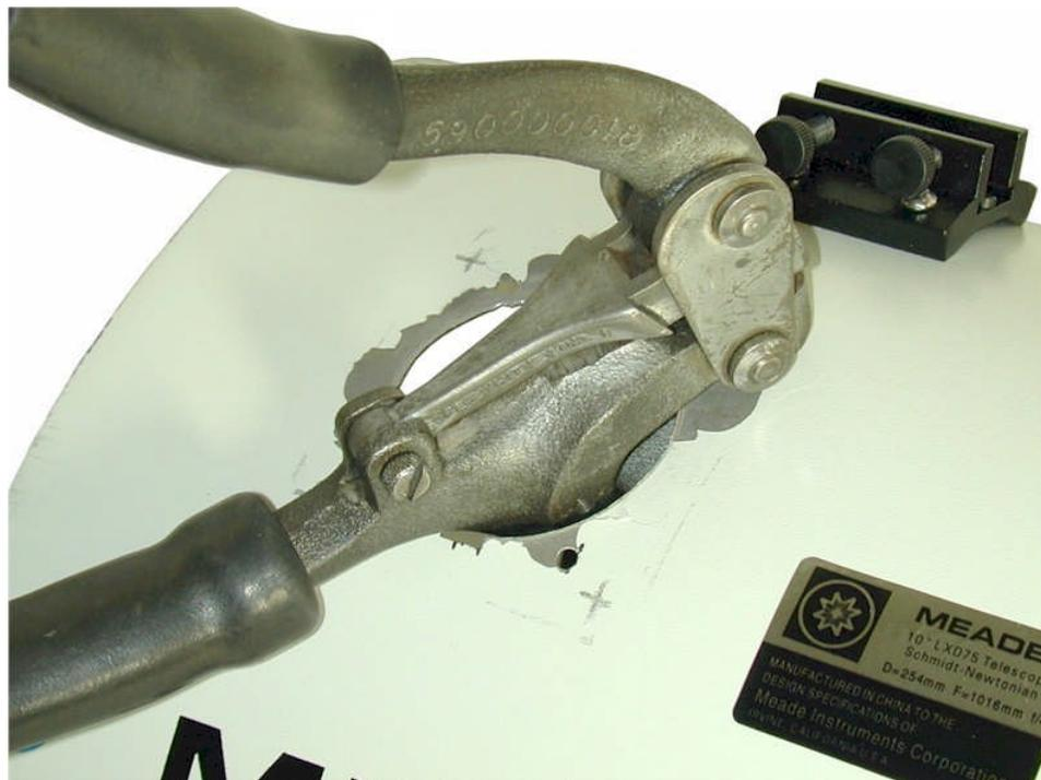
Using a Hand Punch, place four 1/4" holes for the new focuser mounting screws as previously marked.
