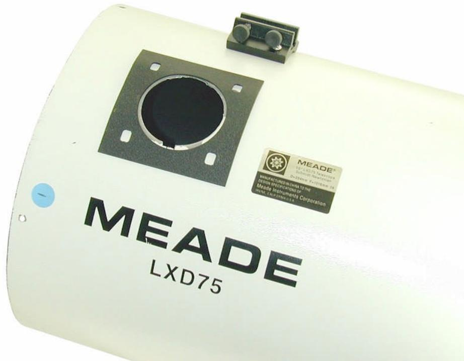
The backup plate will cover the blemishes caused by punching the new hole.
