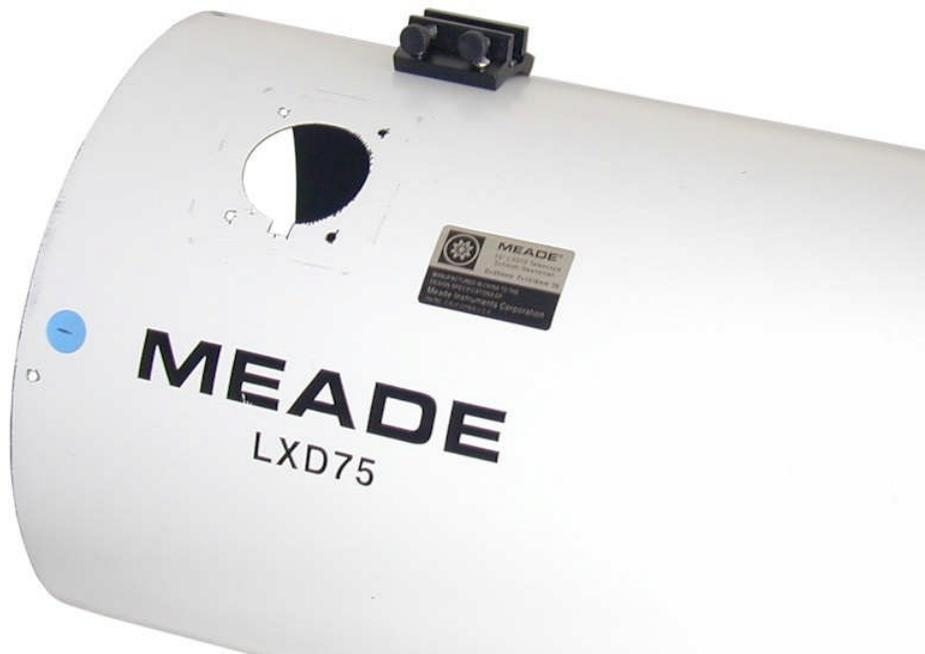
Remove the cover, corrector plate and focuser marking both the corrector plate and the optical tube assembly (see blue sticker in picture) so the corrector plate can be matched up in the same position relative to the optical tube assembly when the job is done.
